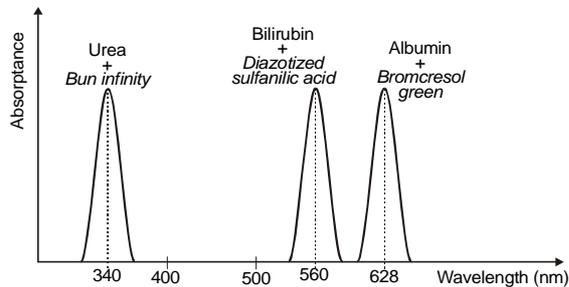
Fig. 4: Absorption spectra shape for urea, bilirubin and albumin.
