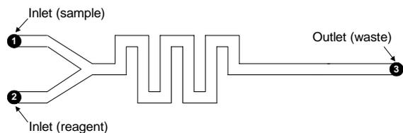
Fig. 2: Schematic top view of the microlaboratory.
