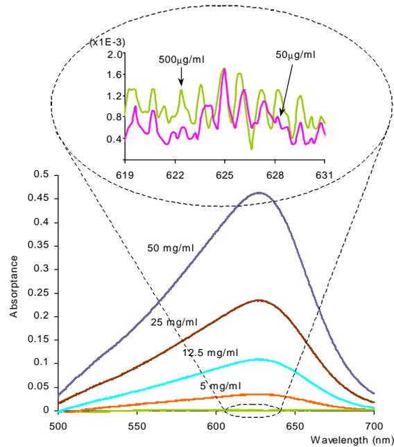
Fig. 5: Absorption spectra for different albumin concentrations, after the binding with bromocresol green.
