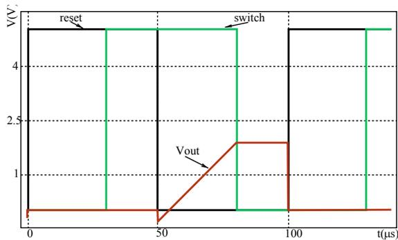
Fig. 10: Transimpedance amplifier output waveform.
