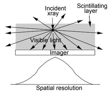
Fig. 1. X-ray imager with a scintillating layer and its spatial resolution.
