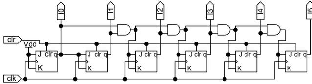
Fig.4: 6 bit counter schematics.
