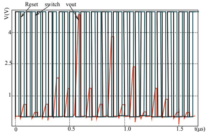
Fig. 11: 8:1 analog multiplexer output waveform for the first 16 pixels.
