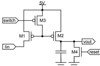
Fig. 9: Transimpedance amplifier circuit.
