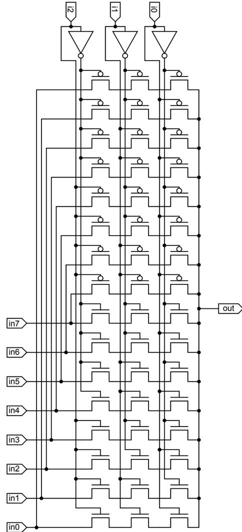
Fig. 7: 8:1 analog multiplexer circuit.
